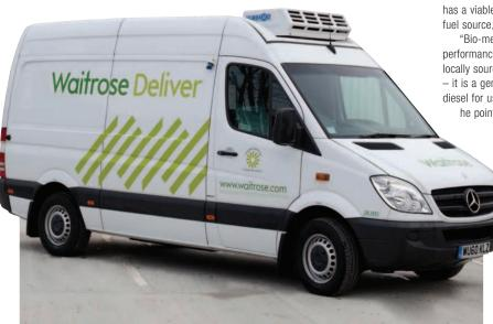
bifuel vehicle, powered by either petrol or gas, with the 1.8-litre, fourcylinder engine delivering 156hp, irrespective of fuel source. As standard, it has a Euro 4 engine, but Waitrose upgrade the power plant to meet the EEV (enhanced environmentally friendly vehicle) emissions standard, above Euro 5.
